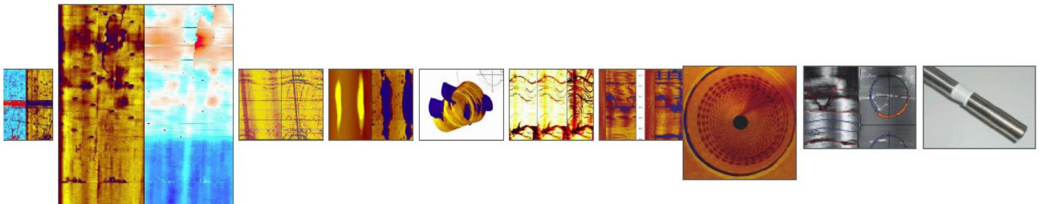
Acoustic borehole scanner tools generate an image of the borehole wall by transmitting ultrasound pulses from a rotating sensor and recording the amplitude and travel time of the signals reflected at the interface between mud and formation (borehole wall).
