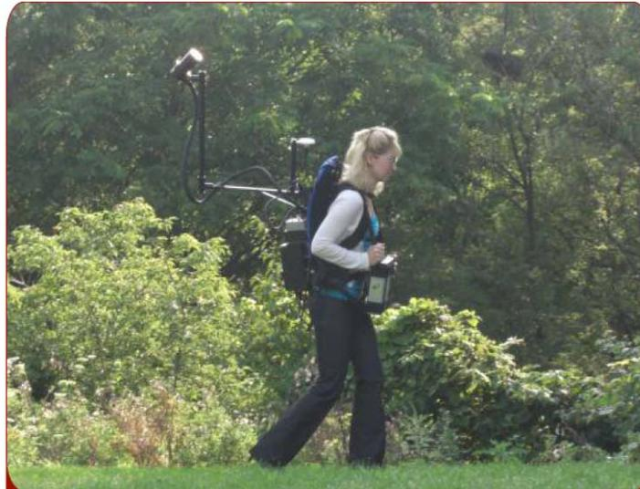
Optically Pumped Potassium (GSMP-40) ground system with backpack, electronics, light weight sensors, and cable.
