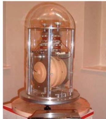
dIdD integrated 3 component coil system with enclosed Overhauser sensor designed for long-term observatory monitoring applications.
