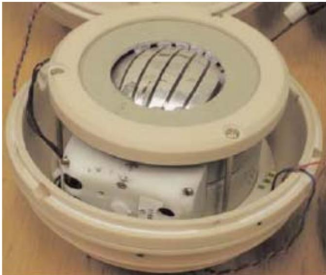
The external casing is impact resistant plastic. An upper support plate ensures that there is no movement of the sensor. The smaller sized sensor has advantages in terms of robustness (i.e. it is more durable than previous generations of larger, cylindrical sensors)
