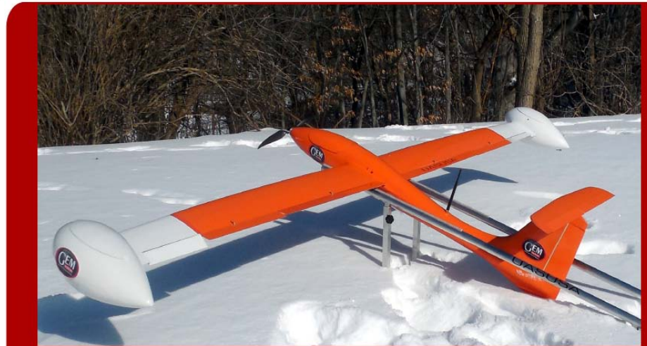
The autonomous GEM MONARCH gradiometer system on its launcher
