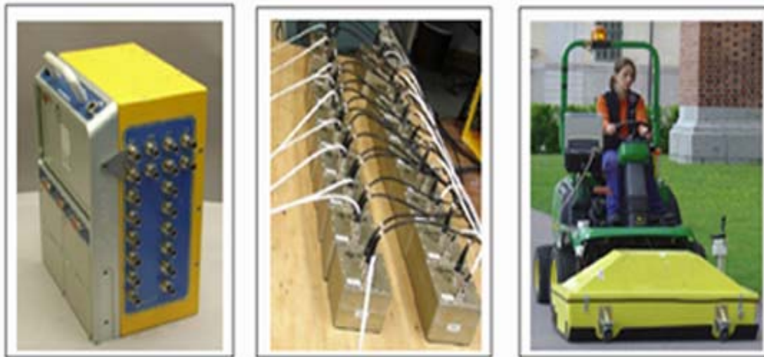
Left: Array option attached to a ProEx control unit. Middle: 1.3GHz Array antennas. Right: Vehicle mounted 400MHz array.
